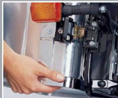
Fit the cases – adjust the mounts if necessary
