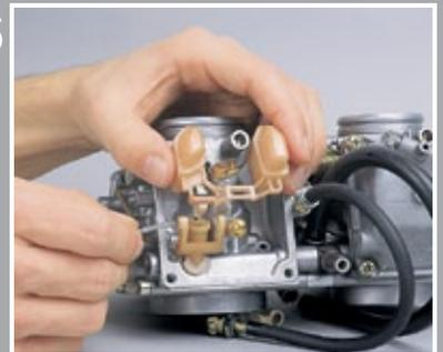
Pull out axle and remove float
