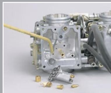
Blow out holes with compressed air
