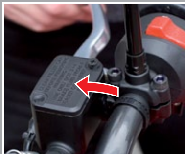
Check cap for correct brake fluid
