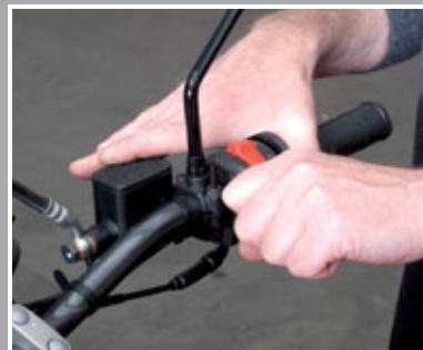
Align brake fluid reservoir horizontally...
