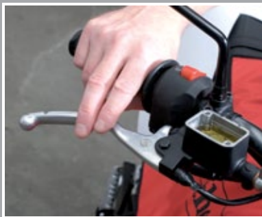
Pump out with brake lever
