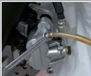
... Fit box-end wrench, attach hose ...
