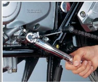
Tighten drain plug with torque wrench
