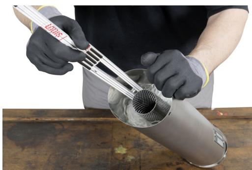
Place the end cap on the silencer so that the perforated pipe is inserted correctly into the socket and the drilled holes for the rivets align again. In the process, use the marking you
