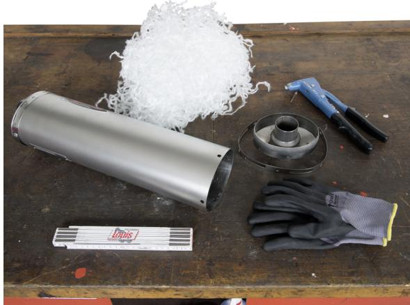
Find a suitable place where you can work cleanly and without interruptions. Lay out your tools and the conversion parts you require. Jack up the motorcycle securely. Make sure that the end cap can be removed from the silencer, e.g. by drilling out the retaining rivets.
