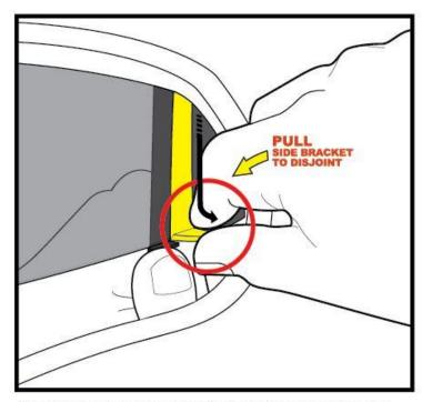
Gently, pry apart the side bracket by pulling the arm towards you to disjoint the bracket from the sun visor. Then release the shield from the clasp, pulling downwards slightly. With one side now disjointed, pry apart the other side to completely detach the sun visor.
