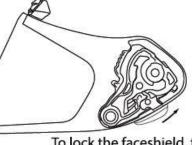
To lock the faceshield, turn Locking-lever counter clockwise to the 2 o'clock position approximately. Check face shield if it's securely locked.
