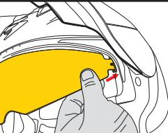
While holding the sun visor firmly, gently pull the sun visor free from its internal housing. Repeat the process on the opposite side. Reverse the process for sun visor installation.
