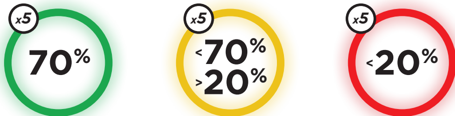
FIGURE 11: EXAMPLE OF FLASHING SEQUENCE INDICATING BATTERY CHARGE LEVEL
