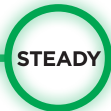
FIGURE 13: SYSTEM ACTIVATED, THE SYSTEM IS READY TO TRIGGER THE AIRBAG.
