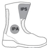
**IPA** = Indicates that the ankle protection (location as illustrated below) has been tested and meets the standard.
