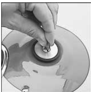
1. Remove left & right pivot discs & screws (You can use a coin)
