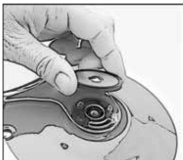
2. Remove the right pivot disc & screw 3. Repeat steps 1 & 2 for left side 4. Remove shield from helmet. 5. Now that the shield is off; the pivot discs will need to be installed back on the helmet in the No Shield position (flush mounted)
