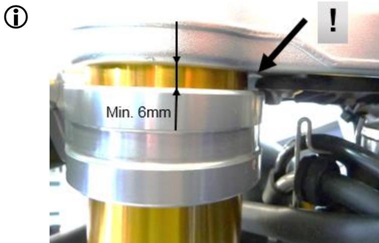
Align Speed Match clamps with bolts M6x25mm about 6mm below the top yoke to avoid a collision to the instruments bracket!
