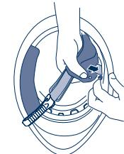
7. Replace the acoustic collar in the guide strip between the bottom edge of the helmet and the high-comfort cheek pads. Start inserting it at the back and slowly feed the acoustic collar along the guide strip.
