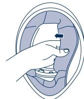
2. Release the high-comfort chin pads by pulling the three red pins out of their plug fittings.
