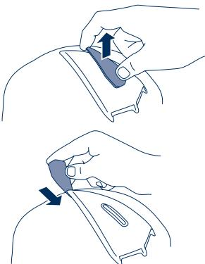
3. On completion of the cleaning, fix the ventilation cowl back in place by hooking it into the front of the ventilation mechanism and pressing it into the helmet shell until you hear an audible click.
