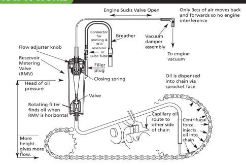
How does the Scottoiler work? The Scottoiler vSystem is vacuum operated. When the motorcycle engine is running vacuum is generated, this lifts a diaphragm which in turn opens the valve. Whilst open the valve allows oil to drip feed under gravity down the delivery tube to the chain via the rear sprocket. There is metering built into the valve to provide adjustment to control the rate at which oil is dispensed. It is not a pump.
