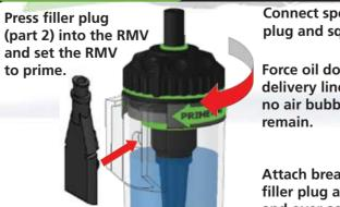
Connect spout to the filler plug and squeeze bottle.
