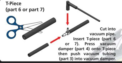
Vacuum tubing & damper elbow **Hint: Lubricate** (part 3 & 4) damper elbow for easier installation.
