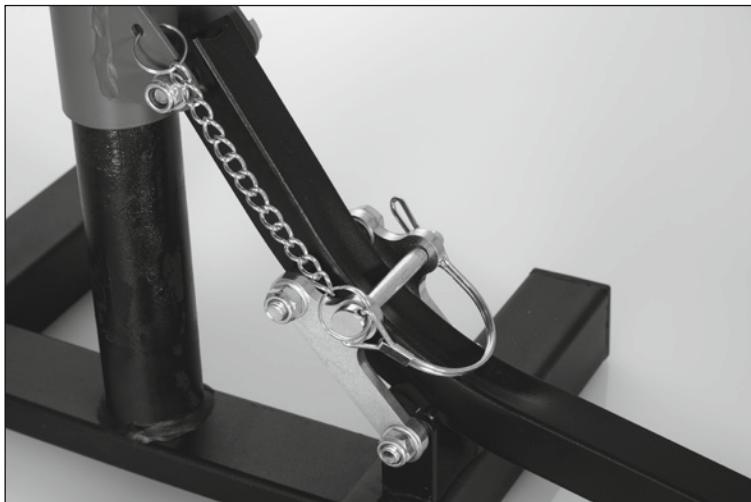
It protects the lever from being shifted back unintentionally, which would cause the motorcycle to fall off/topple over. Flip the bracket safeguard on the locking pin so that the locking pin can slip out of its position.
