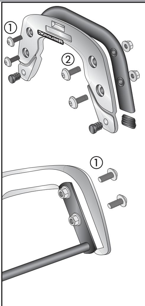
**9** Fastening of the bracing bow and the carrier K-Wing is made in one step.
