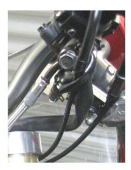
Clutch cable (3): Use the new clutch cable and route it as the original.
