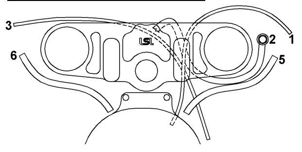
Throttle cable (1): Laying as original. The throttle case has to be mounted with the cables facing downward. Check throttle cable for free movement on every steering angle.
