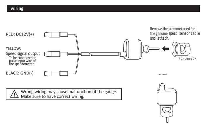
Replace the genuine speed sensor cable with this converter.
