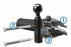
**NOTE:** Both 1/4 in. standard and M6 bolts are included. Match the size of the factory bolts on your clutch-clamp or brake-clamp bracket.
