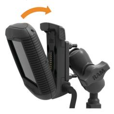
2 Tilt the device back until it snaps into place.
