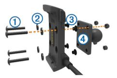
2 Tighten the nuts to secure the base plate.
